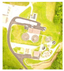
In 1984, the plant capacity was expanded to 700,000 gallons per day, an oxidation ditch installed, 2 clarifiers, a sludge holding tank, and a vacuum sludge drying building were added. Sewer mains were extended to a subdivision of 154 lots near the lake, a recreational campground with 700 lots and extensions to connect across the lake to a proposed commercial development (Tillery Hill). Total cost was \$2.2 million.
